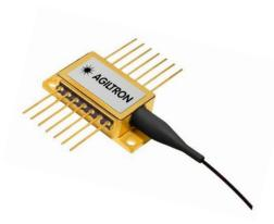
The 945nm series laser diodes are fabricated in a hermetically sealed 14-pin butterfly package. The laser diodes contain a monitor photodiode, thermoelectric cooler (TEC), and a thermistor to secure high-quality laser performance. Our laser products are Telcordia GR-468 qualified and in compliance with RoHS Directives.
